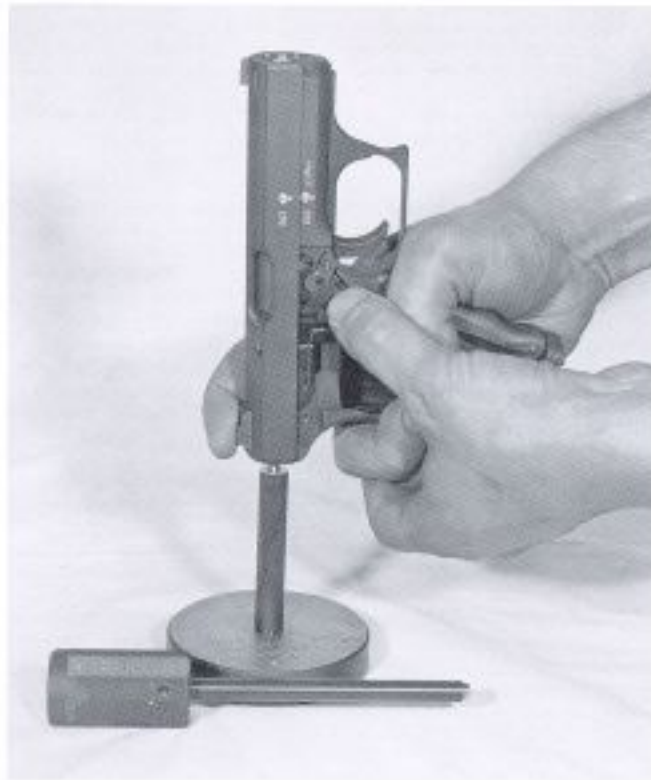
Figure 20. Inspection of firing pin front protrusion.
