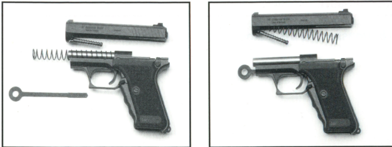
P7 cylinder cleaning tool inserted in the gas cylinder ▲
